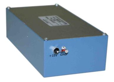
The +15V input terminal is protected with a 1N4746A Zener diode, which will fail as a short if an excessive positive voltage (> 18V), or a negative voltage, is applied to the terminal.
