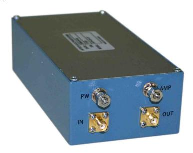
The "AMP" and "PW" controls may be adjusted using a screwdriver.
